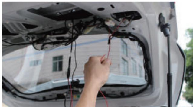
6. Connect the power cord of the rear camera to the front of the car
