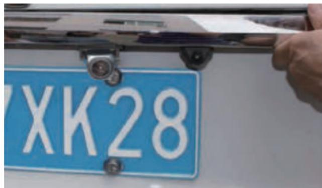
4. Connect the rear lens power cord to the extension cord
